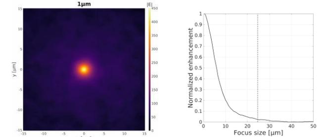
Relationship between enhancement and focus size important for photoacoustic wavefront shaping
