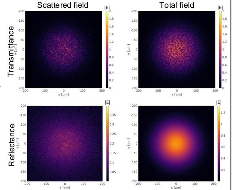
Measurements of **transmittance** and **reflectance** were taken by simulating the propagation of a Gaussian beam through scattering domains.
