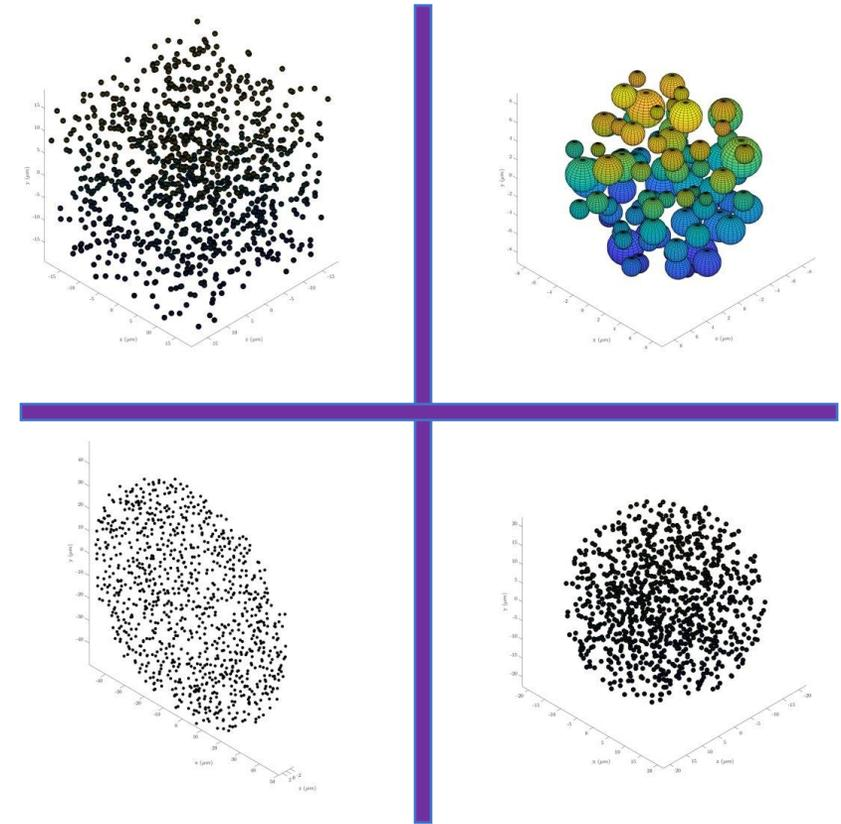
Scatterer refractive index, size and density define bulk optical properties
