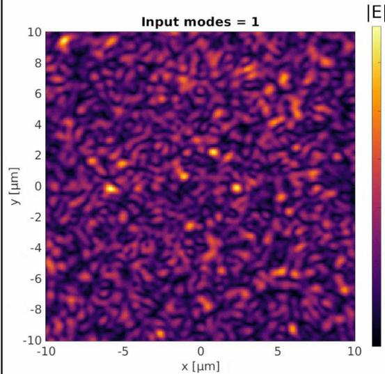
Enhancement is defined as the intensity of the optimized focus to the average intensity of the unoptimized speckle
